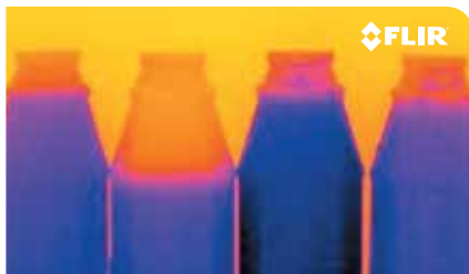
Detecting liquid level in visually opaque bottles.
