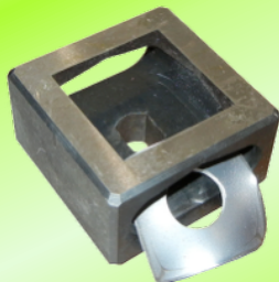
Fig. 2: Slug is ejected out the side of die -- no prying
