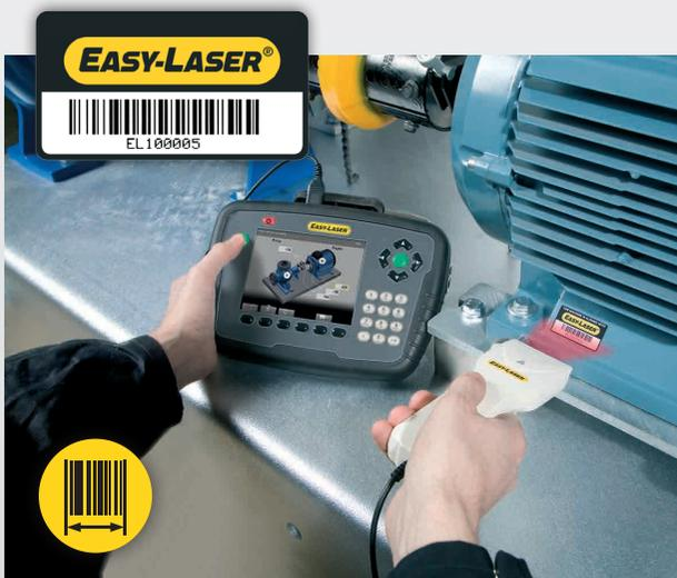
The barcode reader is used to enter the machine data before measurement is taken. After the first measurement is recorded, the adhesive barcode label is applied to the machine. Next time the machine is checked, the measurements, compensation values and tolerances can be read directly from the barcode. Simple and accurate!
