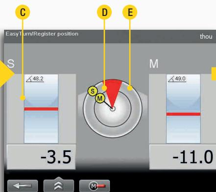
2. Take the measurement values in three positions with as little as 20° between.
