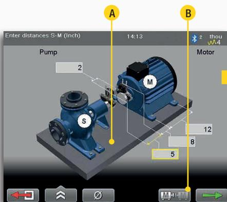
1. Enter the distances between measuring units and the machine feet. If you enter the coupling diameter you can also get the result as gap/sag.
